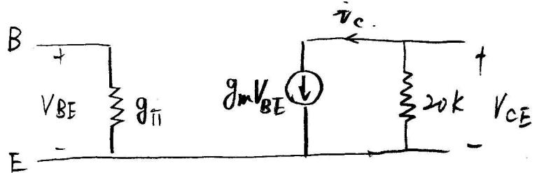
$$\frac{V_{out}}{V_{in}} = \frac{-i_c \cdot R}{V_{BE}} = -g_m R$$
